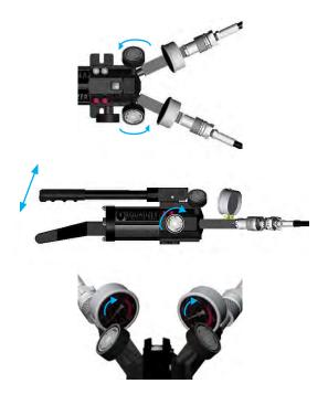
**b.** If control valve 1 is open and control valve 2 is closed with the release valve screwed fully, when the pump handle is raised and lowered only the system connected to control valve 1 will be pressurised (max. 700 bar (10 000 psi)).
